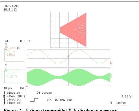
Figure 2 – Using a trapezoidal X-Y display to measure modulation index on an AM signal
