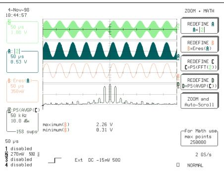
Figure 1–AM signal analysis in the time and frequency domains.
